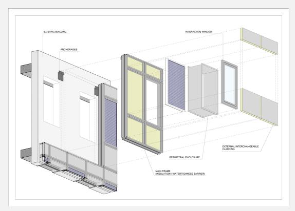
Multiple and alternative modular designs are possible by combining different panels and elements granting significant flexibility and versatility adapted to alternative façade rehabilitation scenarios, with different architectural characteristics, technologies and levels of energy requirements.
