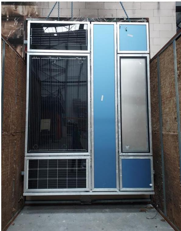
**Figure 7. Full-scaled prototype located in the Fire Test Bench. 6,2 m<sup>2</sup> (Source: TECNALIA)**
