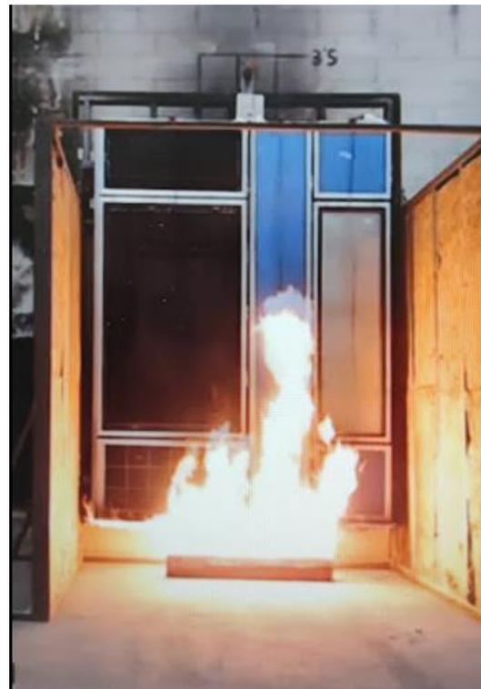
**Figure 8. ISO Fire test being conducted (Source: TECNALIA)**
